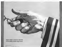
When released, it is energized. Toggle lever stays in opened position, switch remains closed.
